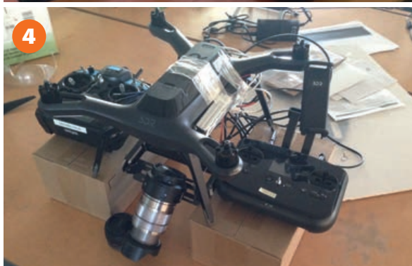
2 to 4 The Solo drone was flying with the GoPro camera however, Dan McKinnon was keen to use a new QX-1 camera from Sony and so prototyped a contraption that connects this camera via software and hard cable to the Solo
