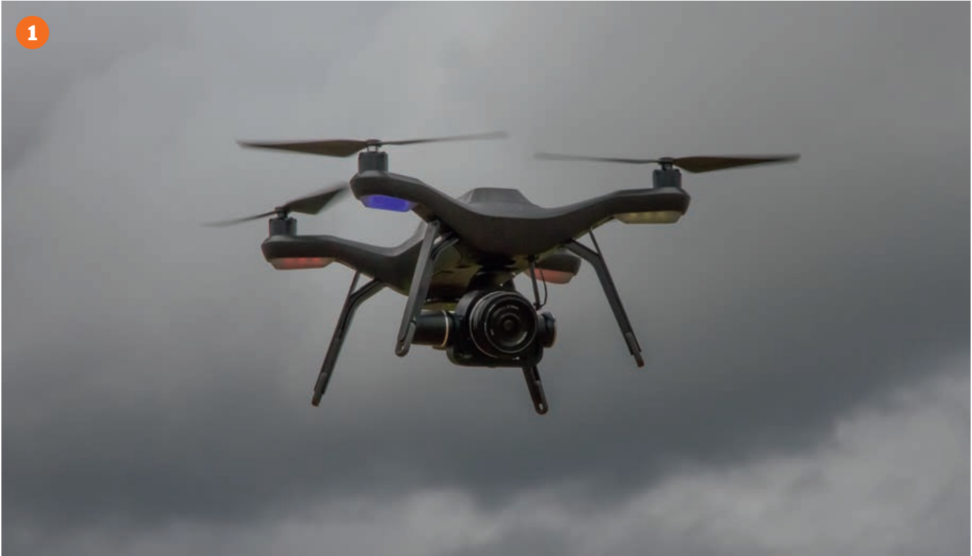
1 The Solo drone collects high-quality data with the Sony UMC-R10C camera
